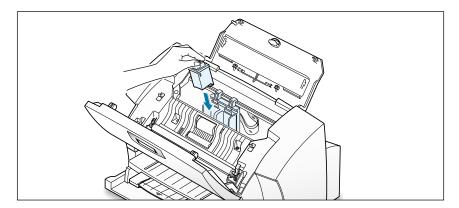
7. Push the cartridges back until the cartridge locks firmly into place.
